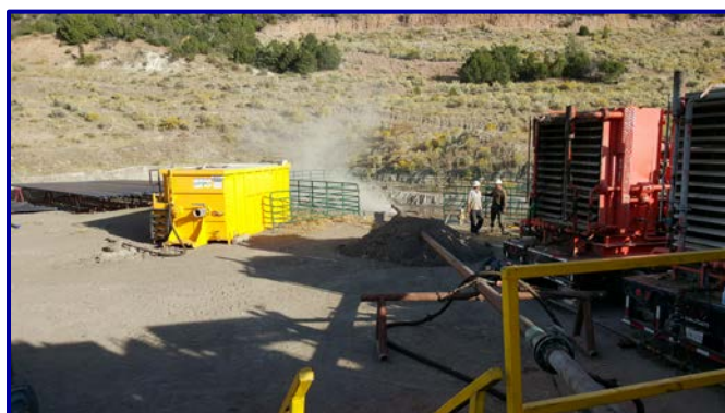
Drill cuttings being returned to the drilling pits under pressure through the blooie line
